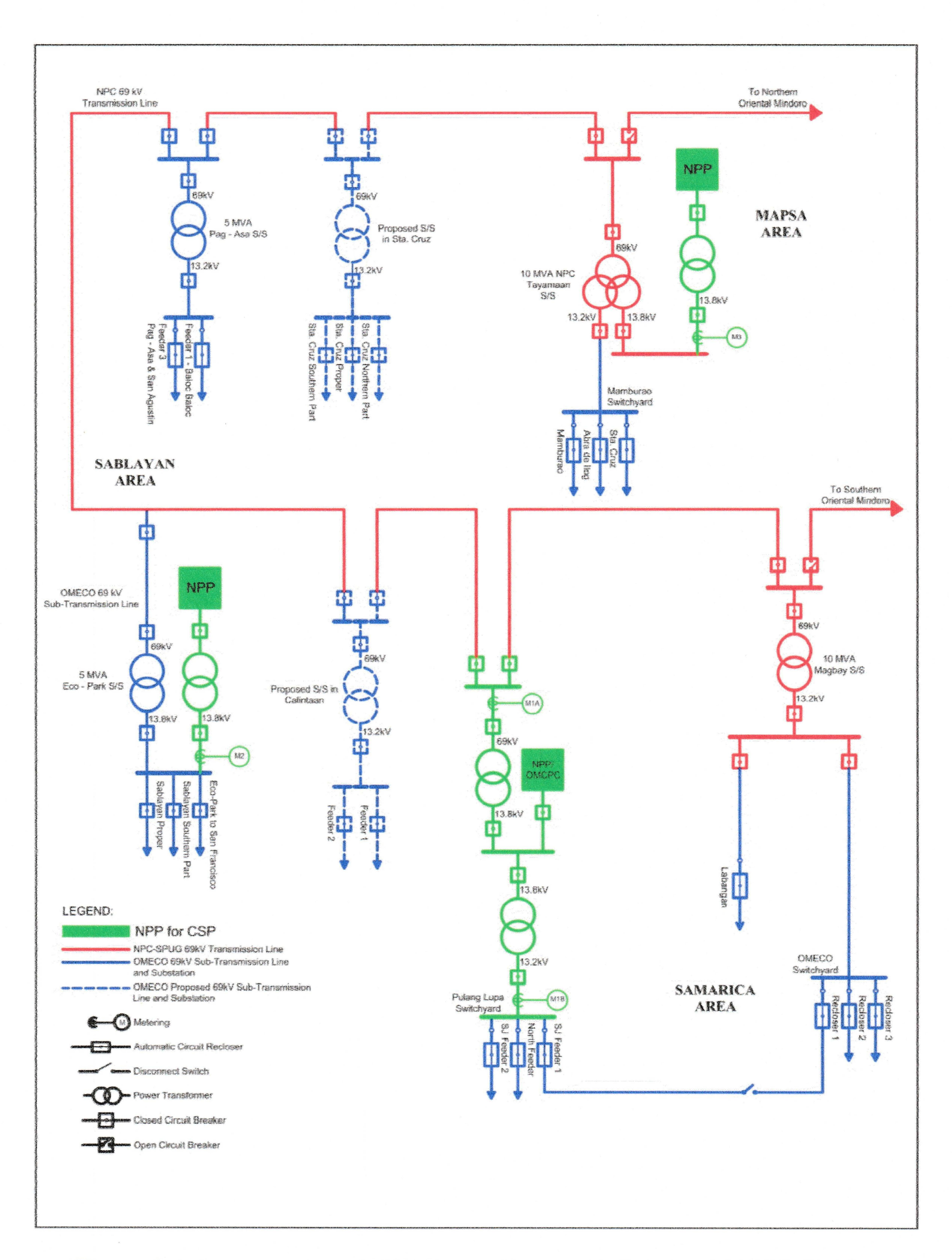
Figure 2: Interconnection of NPP Power Plants with Existing OMCPC Plant at SAMARICA
